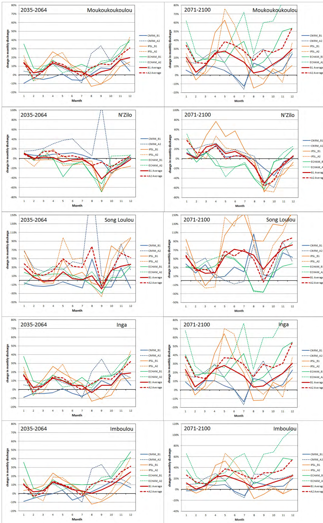
Figure 14. Relative changes in river flow into hydropower reservoirs for five different dams in Central Africa for mid 21 st century (left panel) and the end of the century (right panels). Each line (except red) shows the result of an individual climate model. Red lines show the average of the three different climate models. Dashed lines indicate a high emission scenario (A2) and straight lines a low emission (B1) scenario.
